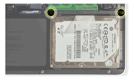
**7** To prevent strain on hard drive cable, disconnect cable from logic board and remove 3-mm long screw.
